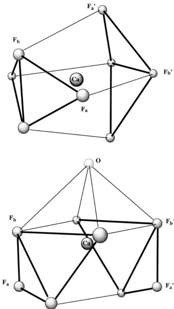
**Fig. 2** The dodecahedral (a) (top) and approximate tricapped trigonal prism co-ordination geometry (b) (bottom) of complexes **2** and **4**, respectively. The co-ordinating fluorine atoms ( $F_a$  and  $F_b$ ) of each  $[\text{Ti}_2(\text{C}_5\text{Me}_4\text{Et})_2\text{F}_7]^-$  moiety are connected by bold lines.
