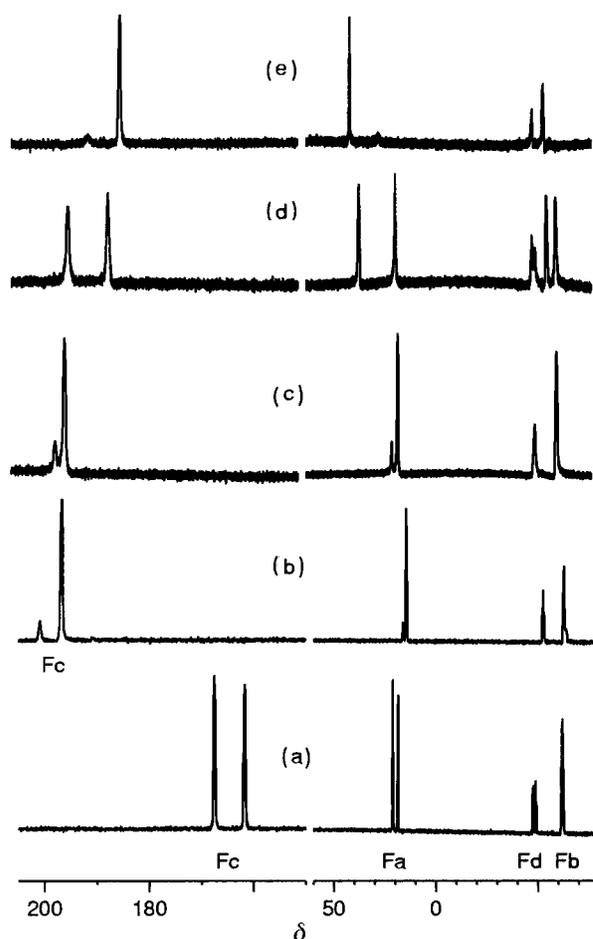
**Fig. 3** The  $^{19}\text{F}$  NMR spectra of calcium fluoride complex **2** in (a)  $\text{CDCl}_3$ , (b)  $[\text{C}_6\text{D}_6][\text{H}_8]\text{thf}$ , (c)  $\text{C}_6\text{D}_6$ , (d)  $\text{C}_6\text{D}_6-[\text{C}_6\text{D}_6][\text{H}_8]\text{thf}$  (20:1) and (e)  $\text{C}_6\text{D}_6-[\text{C}_6\text{D}_6][\text{H}_8]\text{thf}$  (2:1). See Scheme 1 for labels.
